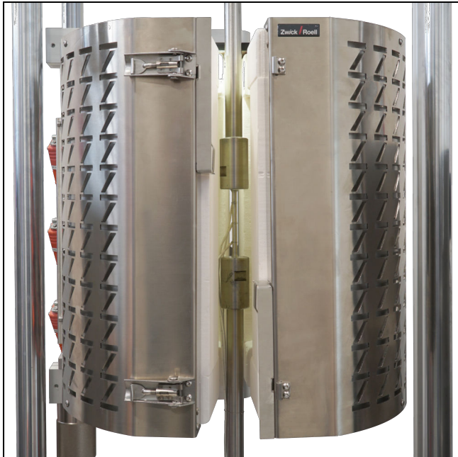
1,200 °C high-temperature furnace with three heating zones
