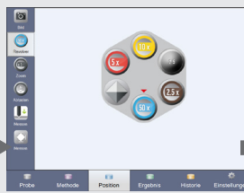
The turret shows the currently swiveled-in objective or indenter
