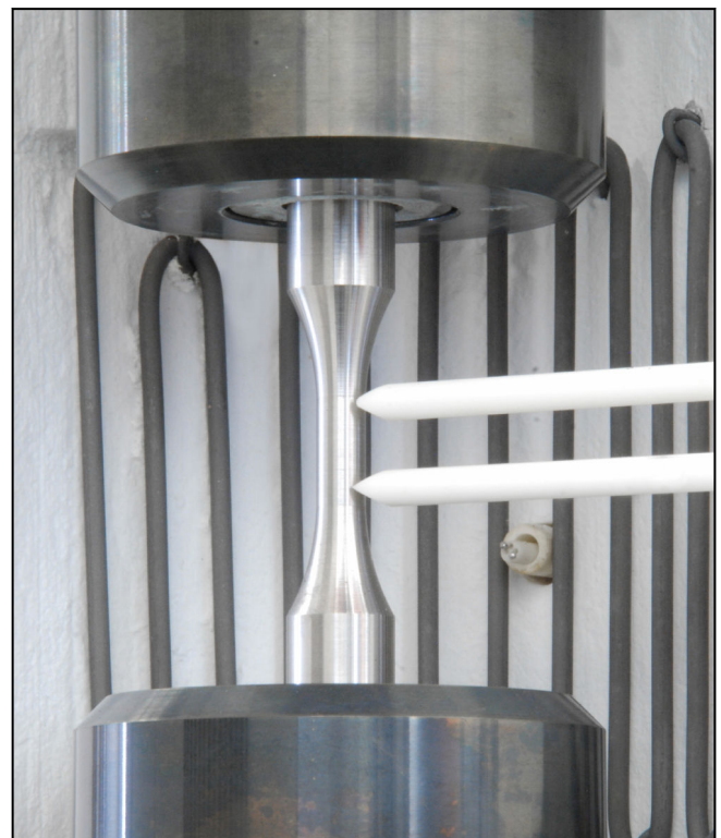
Specimen plus extensometer in high-temperature furnace
