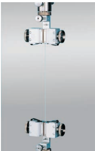
Fig. 3: Wedge-screw grips 500 N
