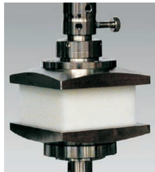
Fig. 3: Foam testing with compression platen 120 x 120 mm
